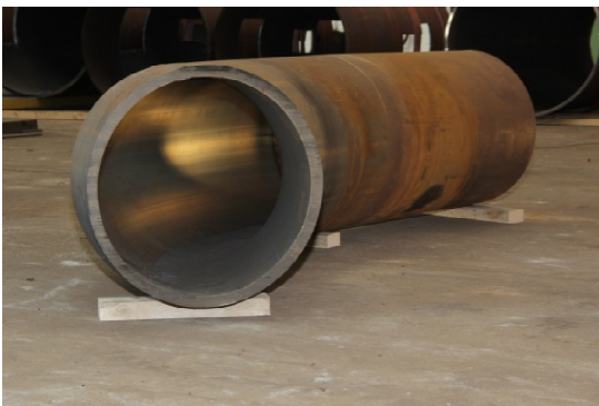
Figure 8: 3D Clad Bend, 24" x 42mm WT
