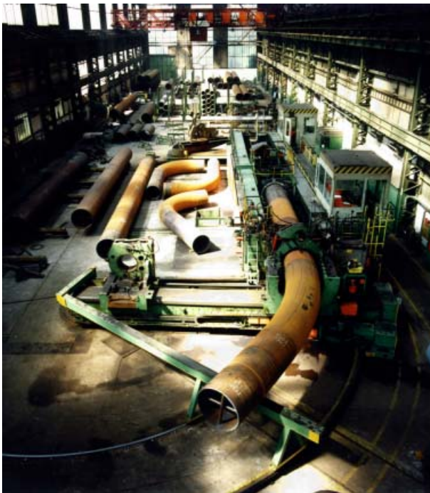
Figure 1: Hot induction bending of 48” line pipe at Mannemmann Bending Plant
