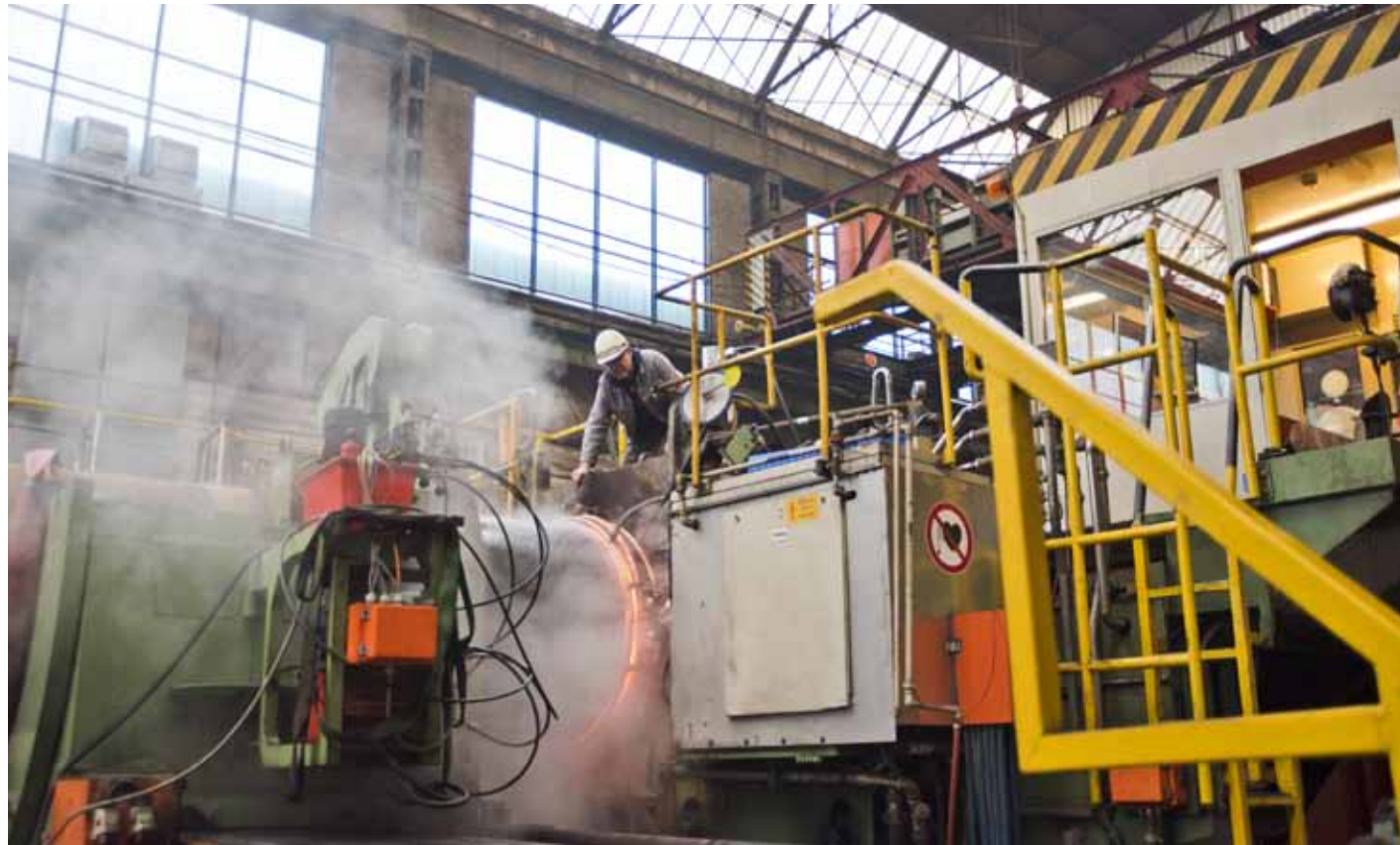
The pipes are shaped by way of induction bending at the pipe bending mill – completed in a wide range of angles
