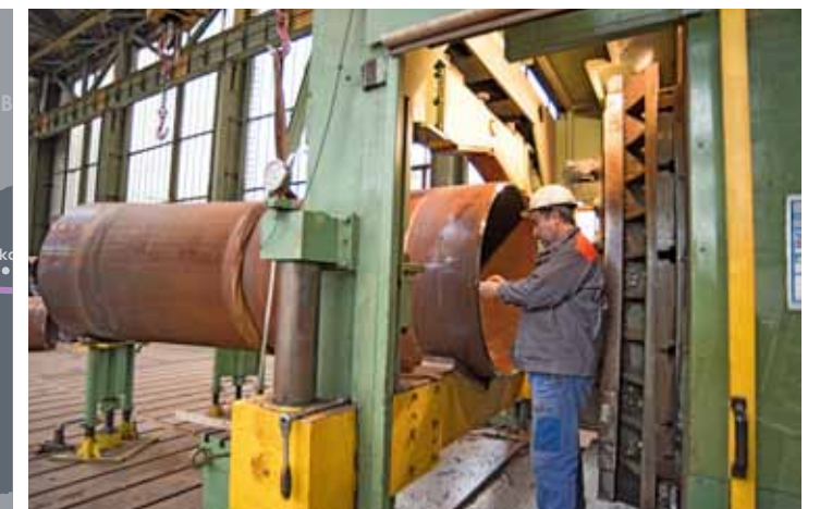
Each end of a pipe bend is machined and supplied with a welded bevel. The geometry has to be just right to avoid any problems on the building site in circumferentially welding the pipe bends with the line pipes
